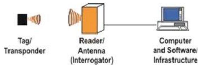
Figure 2.1: Basic components of RFID system [1]
